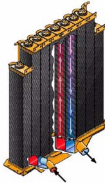
Figure 27 - Caterpillar AMOCS Radiator and Coolant Flow
