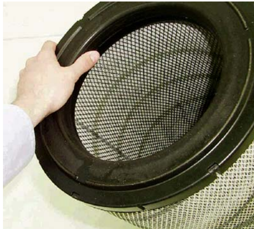
Figure 17 - Dry Element Cleaning
