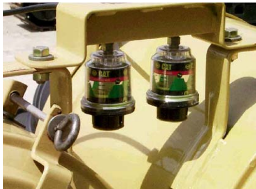
Figure 19 - Typical Twin Air Cleaner, each with its own Service Indicator
